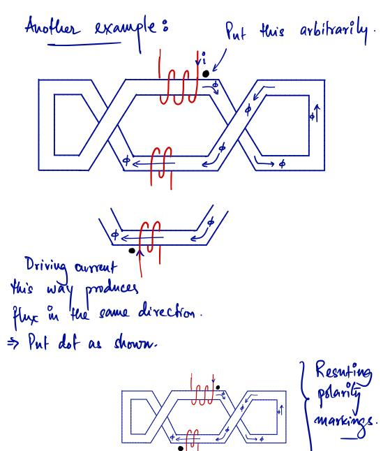
2 Deriving circuit equations or loop equations, given polarity markings. tollow the rule below:-Voltage difference )
